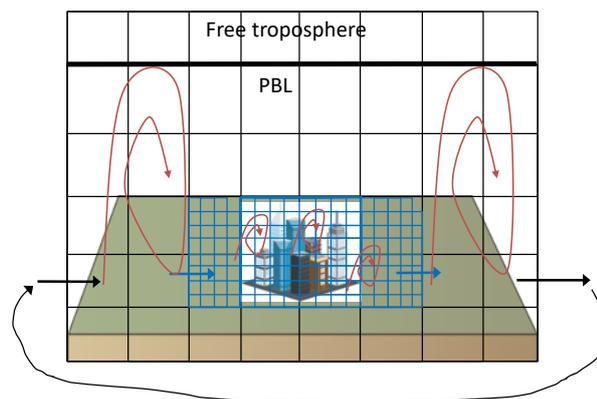
Figure 1. A notional depiction of the nested grid approach used in JOULES.
