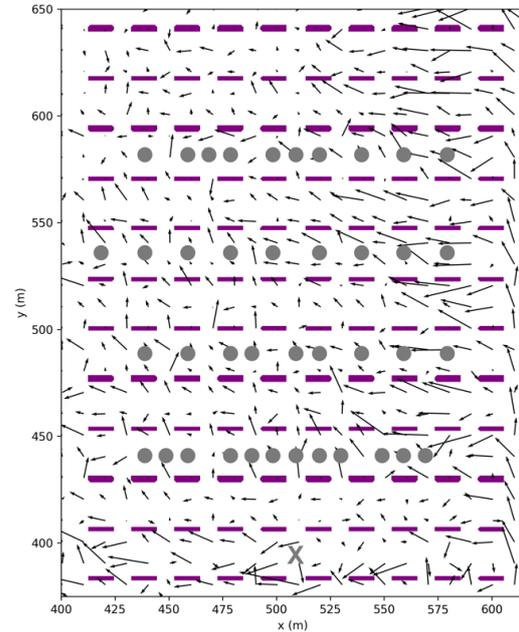
Figure 3. A depiction of the simulated MUST obstacle array (purple rectangles), propylene sensor locations (grey filled circles), release location (grey X), and near surface wind vectors.
